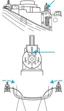
Turning the horizontal adjusting screw in the direction of the arrow changes the horizontal aim as shown.
